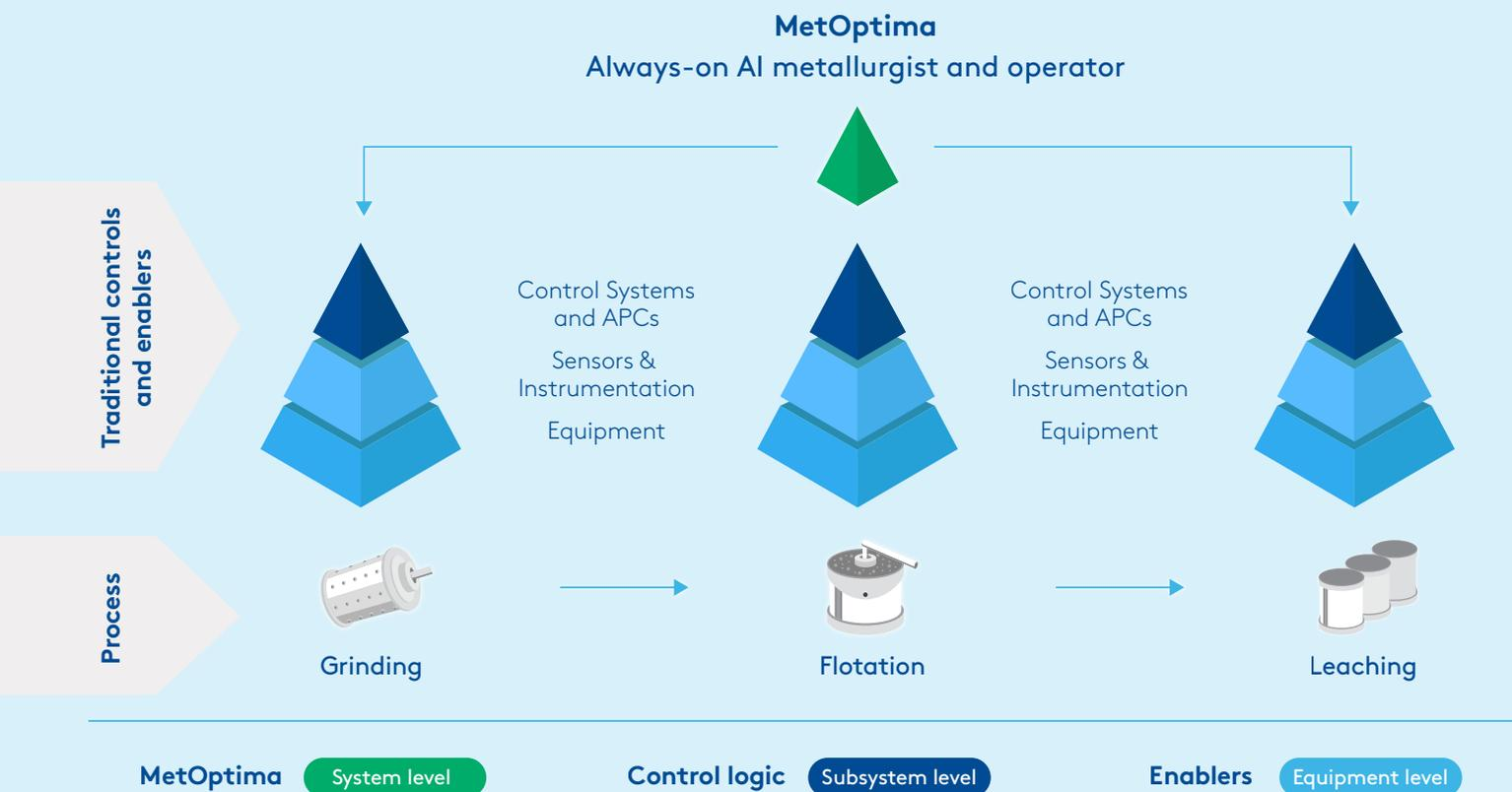
It leverages aggregated plant and sensor data through the client adapter and applies our suite of advanced analytical and predictive models to the data to generate recommendations every 4 hours, which the shift operator either accepts or rejects via a user-friendly web app.
